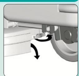
**CLEAN THE INNER FILTER OF THE SOLUTION TANK:**
