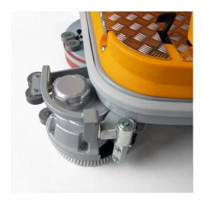
The side brush is <u>an optional</u> and it has to be ordered separately from the machine, but in any case when ordering, because the retrofit is not so easy.
